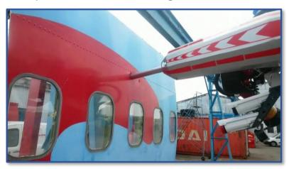
Harder; Longer & Deeper with the CHINETTI HRET fully proportional hardened steel tip Fuselage Penetrator with nozzle for rapid media deployment inside the aeroplane, utilising Ultra Motion Technology and Hydraulic Battery power
